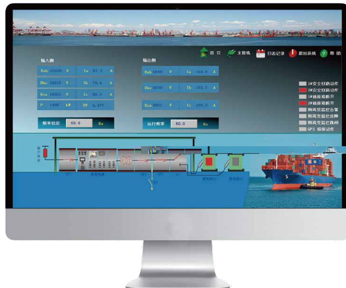
Shore Power Monitoring System
